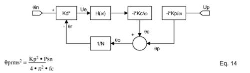
Kp is the pushing coefficient of VCO, Psn is the noise power of the power supply, fc is the 3dB corner frequency of the PLL filter.
