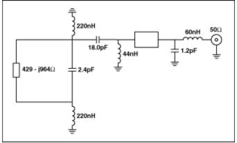
Figure 7. Final design uses 3 capacitors.
