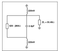
Figure 5. Design is tuned to resonate at 183.6 MHz with 220 nH inductors.
