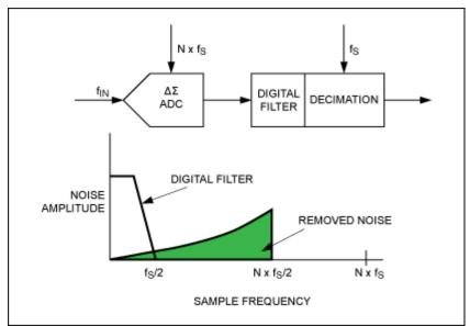
Figure 3. ADC with oversampling by factor of N, noise shaping, digital filter, and decimation. Noise (green area) in the ADC's input frequency band of interest becomes very small.
