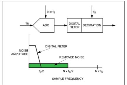
Figure 2. ADC with oversampling by a factor of N, digital filter, and decimation.
