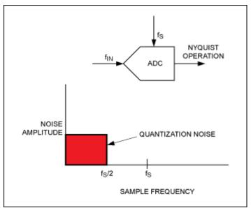
Figure 1. Standard ADC noise performance.
