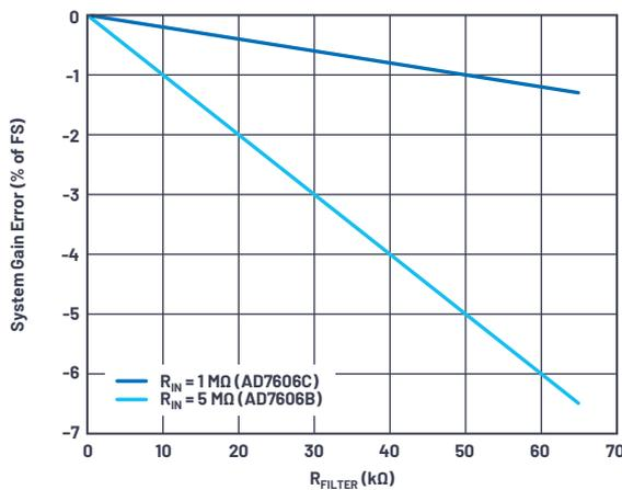
Figure 8. System gain error (% of FS) comparison depending on input impedance ( $R_{IN}$ ).
