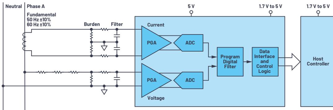
Figure 1. A typical signal chain in power monitoring applications. Only one phase is shown for simplicity.
