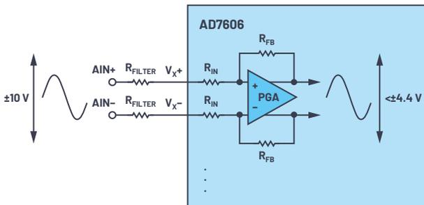
Figure 4. A series resistor in front of the AD7606's analog inputs ( $V_{X+}$  and  $V_{X-}$ ) modifies the system gain.
