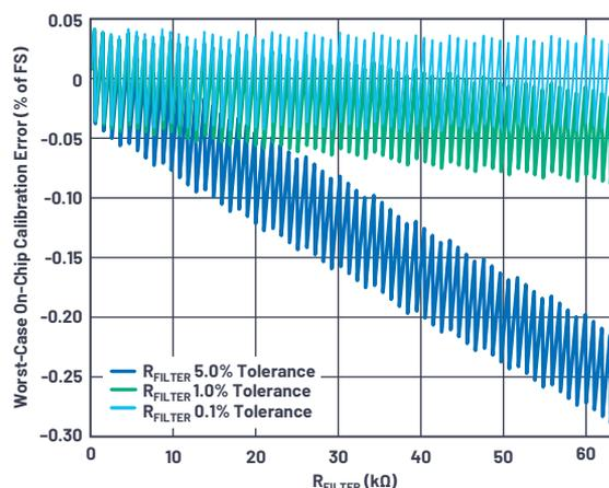
Figure 13. Impact of  $R_{\text{FILTER}}$  discrete resistor tolerance on the on-chip calibration feature accuracy (worst-case scenario).
