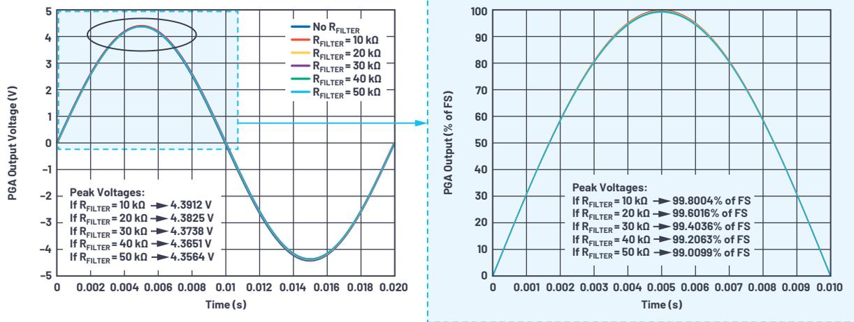
Figure 7. AD7606B's PGA output amplitude is less impacted by the external  $R_{FILTER}$ , because of the higher input impedance (5 MΩ).
