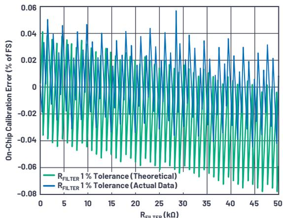
Figure 16. Actual AD7606C-16 results compared to theoretical analysis.
