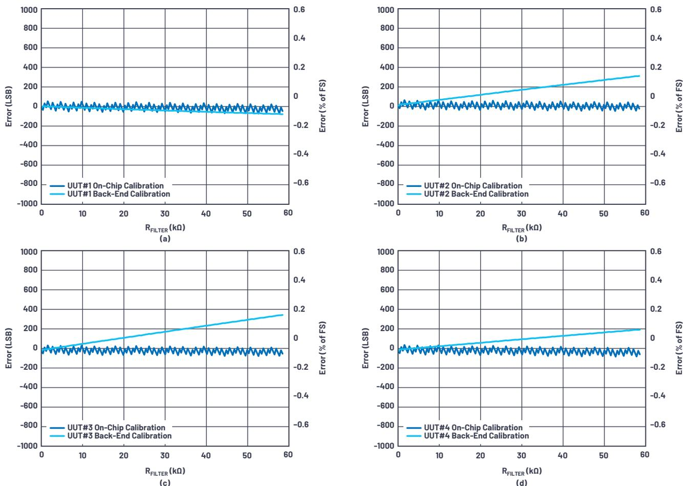
Figure 17. Comparison between on-chip calibration and back-end calibration across four AD7606C-18 units.
