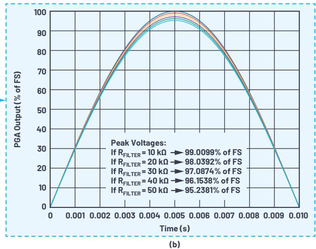
Figure 5. The PGA output's amplitude decreases with the size of the  $R_{FILTER}$ . (a) Shows the PGA output voltage in volts and (b) shows the PGA output voltage as a percentage of FS.
