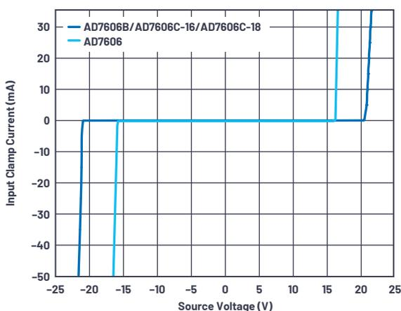
Figure 2. AD7606 input protection clamp profile.
