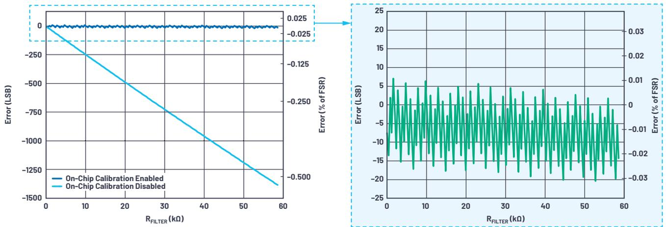
Figure 15. (a) System gain error as a function of  $R_{FILTER}$  for the AD7606C-16 with and without enabling the on-chip gain calibration and (b) close-up of the on-chip calibration plot.
