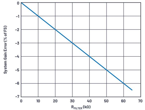
Figure 6. System gain error (% of FS) as a function of the external  $R_{FILTER}$  resistor in AD7606 (1 MΩ input impedance).
