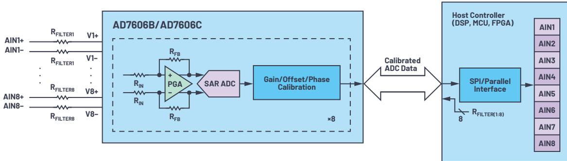
Figure 11. On-chip calibration blocks. Only one channel is shown as an example.
