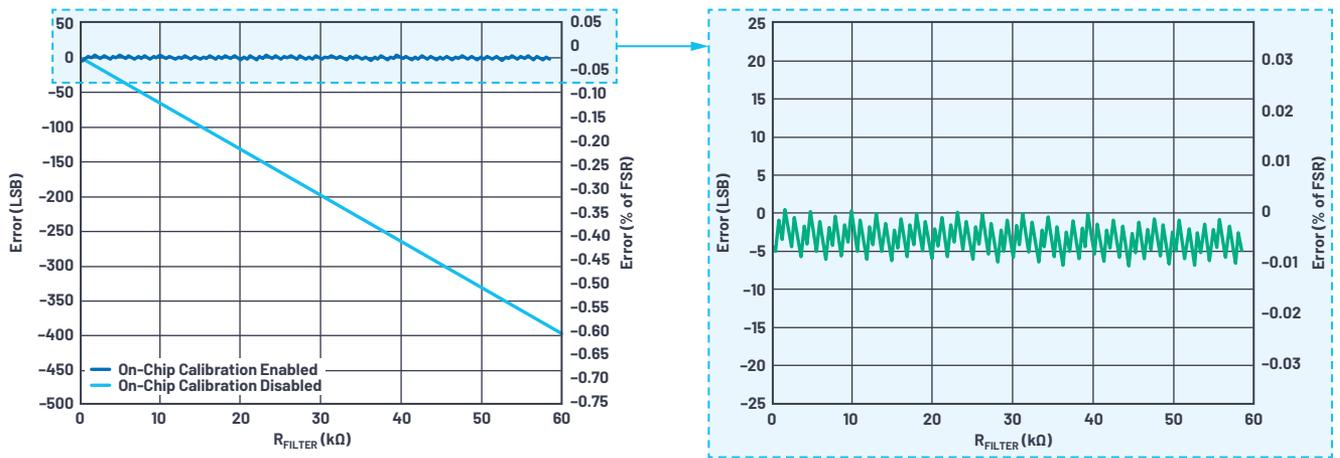
Figure 14. Total error of the AD7606B with the on-chip gain calibration enabled.
