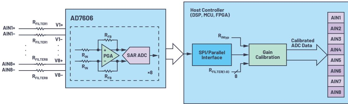
Figure 9. Back-end calibration blocks. Calibration is done on the host controller assuming typical value for  $R_{IN}$  and knowing the external resistor value  $R_{FILTER}$ .
