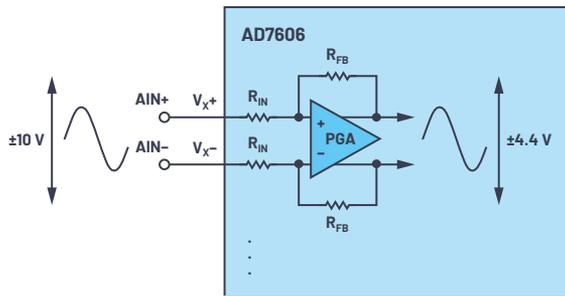
Figure 3. AD7606 internal PGA. Only the ±10 V range is shown as an example.
