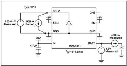
Figure 7. Measuring forward voltage for the MAX1811 ESD diode in normal operation. Testing the MAX1811 Thermal-Control Loop
