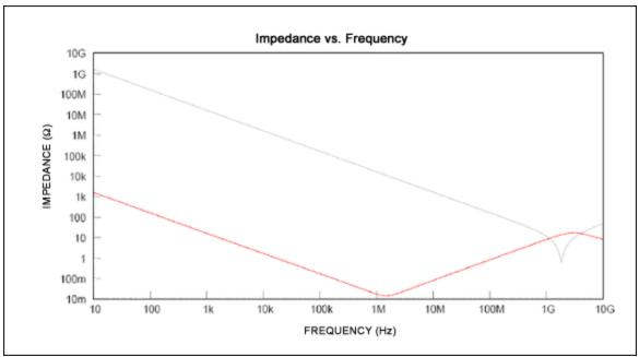
Figure 1. RF signals can be picked up by the amplifier's power supply connections. The above data show that the  $1\mu$ F capacitor offers lower impedance to ground than the 10pF capacitor, thus providing better noise suppression.
