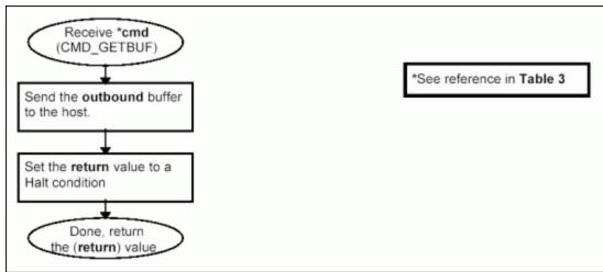
Figure 3f. Processing command CMD\_GETBUF.
