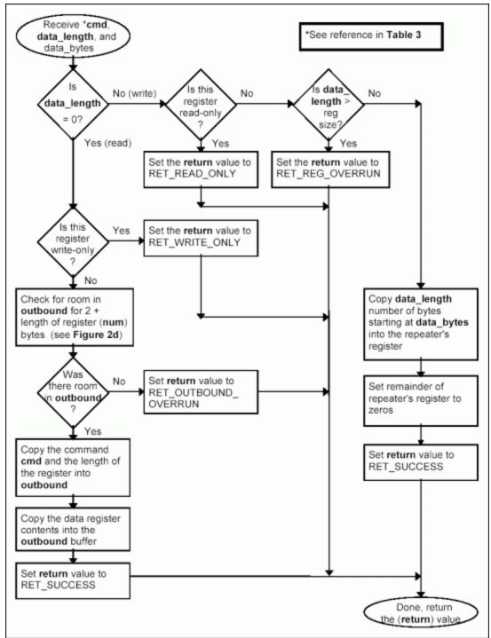
Figure 3g. Processing data register commands.
