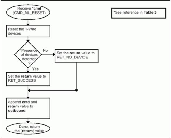
Figure 3a. Processing command CMD\_ML\_RESET.
