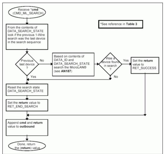
Figure 3b. Processing command CMD\_ML\_SEARCH.
