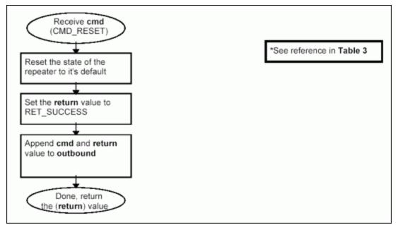
Figure 3e. Processing command CMD\_RESET.
