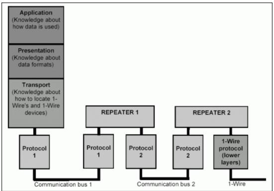
Figure 1. Repeater in a multiple-protocol scenario.
