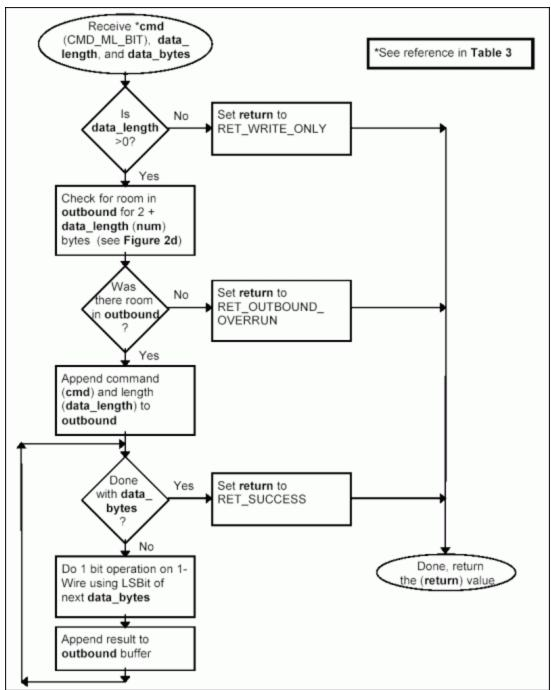
Figure 3h. Processing command CMD\_ML\_BIT.
