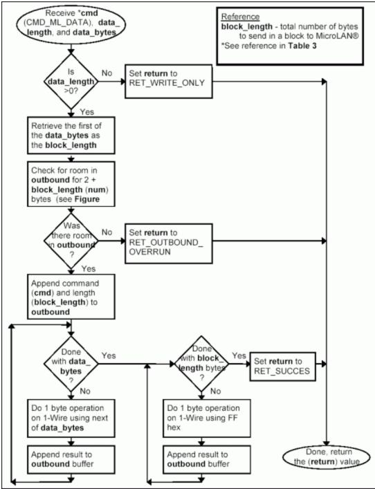
Figure 3i. Processing command CMD\_ML\_DATA.
