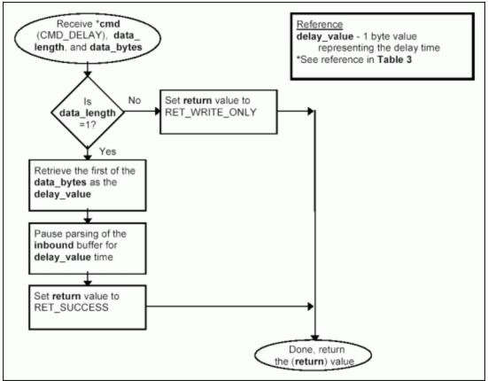
Figure 3j. Processing command CMD\_DELAY.
