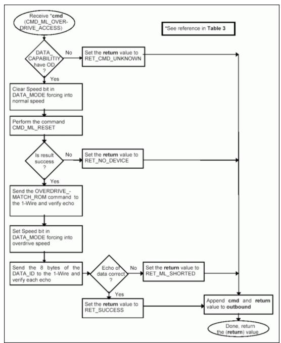
Figure 3d. Processing command CMD\_ML\_OVERDRIVE\_ACCESS.
