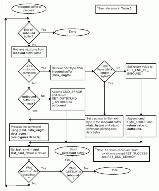
Figure 2b. Inbound command processing.
