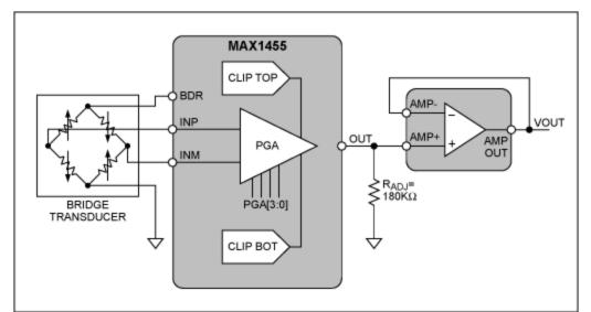
Figure 4. Intentionally pulling the clip voltage off set value and to a new desired value with R<sub>ADJ</sub>.
