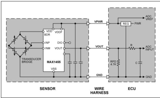
Figure 2. Typical sensor wiring configuration.
