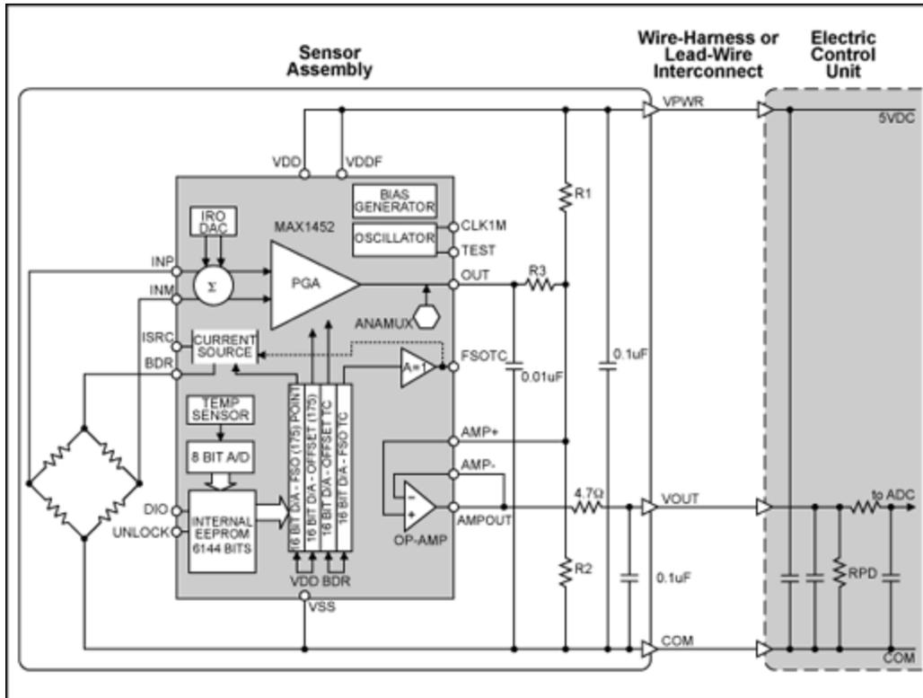
Figure 3. Typical sensor wiring configuration.
