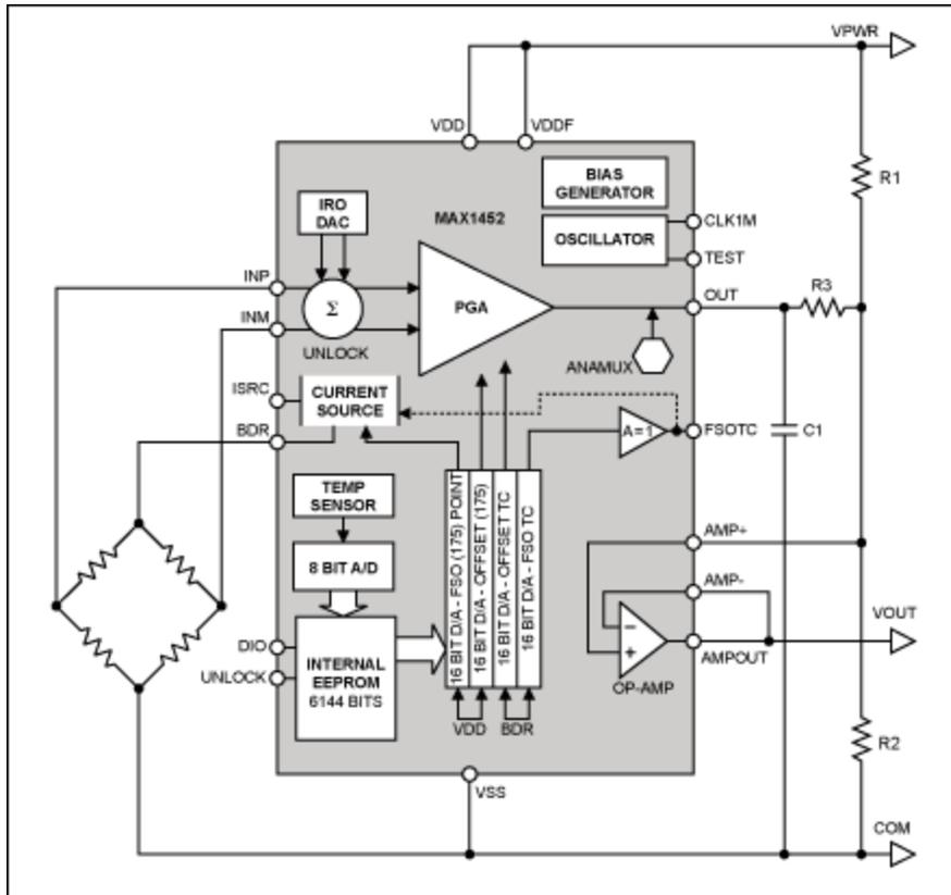
Figure 4. Creating clip-high and clip-low diagnostic voltage limiting.
