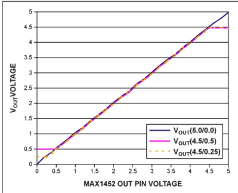
Figure 2. Various output diagnostic clip settings.
