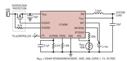
Figure 1. The LTC4099 with I<sup>2</sup>C controlled battery conditioner
