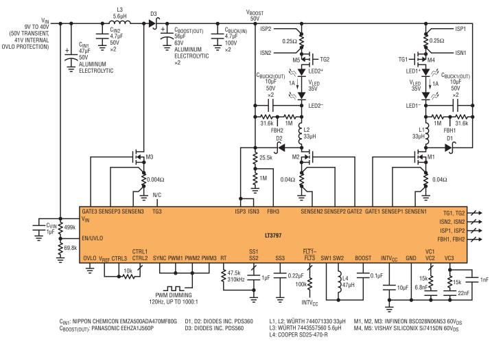
An extra benefit of the boost-then-buck mode driver is the reduced conducted EMI versus a similarly rated buck-boost regulator. Boost converters typically have lower conducted EMI around the AM band than buck converters due to the location of the main inductor in series with the input. In a boost-then-buck scheme, the inductor is in series with the input, versus a buck-boost single inductor between the buck and boost stages.
