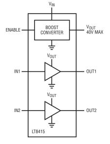
Figure 1. Simplified block diagram of the LT8415
