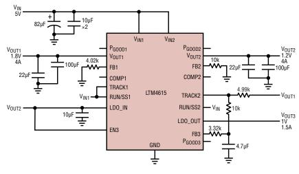
Figure 11. Output voltage tracking design example
