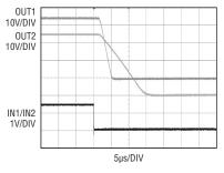
Figure 4. Turn-off delay and fall time for OUT1 and OUT2
