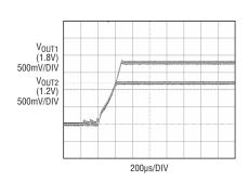
Figure 12. Start-up waveforms for the circuit in Figure 11
