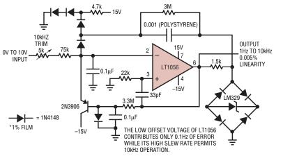
Figure 1. Precision: 1Hz to 10kHz voltage-to-frequency converter
