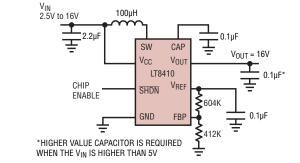
Figure 1. 2.5V-16V To 16V boost converter
