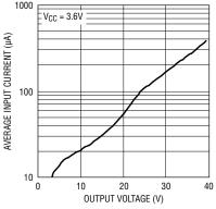
Figure 6. Average input current in regulation with no load
