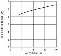
Figure 5. Quiescent current vs V<sub>CC</sub> voltage (not switching)
