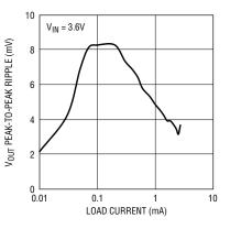
Figure 3. Output peak-to-peak ripple vs load current for Figure 1 converter at 3.6V
