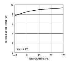
Figure 4. Quiescent current vs temperature (not switching)
