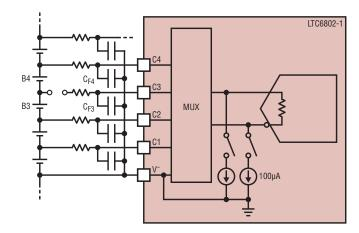
Figure 11. Current sources help detect open circuits.
