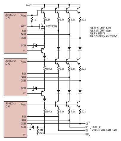
Figure 14. Inexpensive SPI daisy chain for parallel-addressed LTC6802-2
