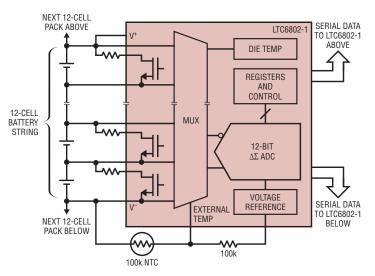
Figure 4. Simplified block diagram of the LTC6802
