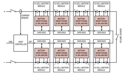
Figure 1. 96-cell battery pack
