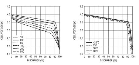
Figure 3. State of charge vs current and temperature for a typical Li-ion cell
