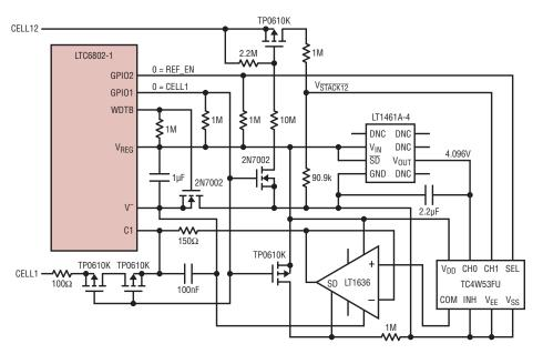
Figure 7. Improving accuracy with calibration
