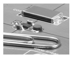
Figure 1. A complete PCMCIA-powered, low profile solution for GSM transmitters
