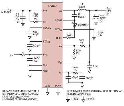
Figure 1. Typical application of the LTC3608
