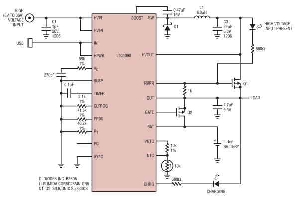
Figure 1. Li-Ion battery charger accepts both USB and high voltage inputs
