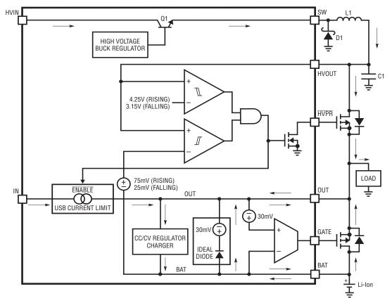
Figure 3. Simplified block diagram of the LTC4090 PowerPath operation
