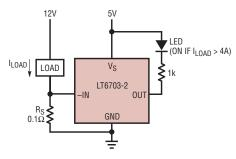
Figure 5. Low side current sense alarm
