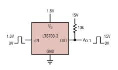
Figure 4. Simple level translator for shifting low voltages to high voltages
