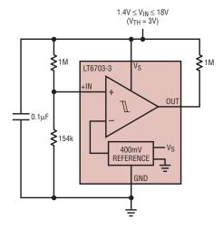
Figure 2. Micropower supply voltage monitor
