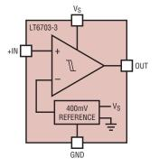
Figure 1. Block diagram of tiny 2mm × 2mm 1.4V-to-18V comparator
