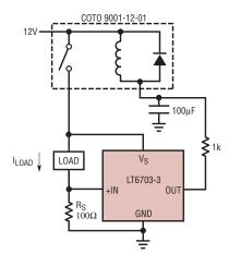
Figure 6. Latch-off protection circuit
