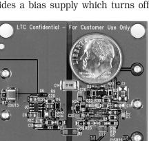
Figure 2. Isolated 36V to 72V to 3.3V 3A flyback converter
