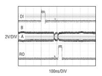
Figure 8. The LTC2854 driver delivering a single 50ns pulse through 100ft of Cat 5 cable, which is received by another LTC2854. Both parts have their on-chip termination enabled. Top trace is the input to the transmitting device and the middle and bottom traces are observed at the receiving part.
