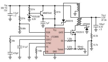
Figure 1. Non-isolated 36V to 72V to 3.3V 3A flyback converter
