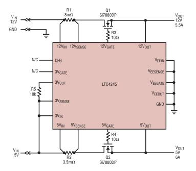
Figure 8. A 12V and 5V application. Floating the CFG pin disables the  $V_{EE}$  undervoltage and power bad functions, allowing those pins to be tied to GND.
