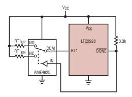
Figure 5. Active sequence positioning using an analog multiplexer
