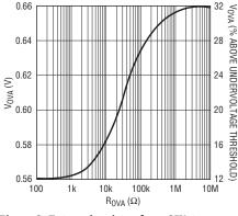
Figure 3. External resistor from OVA to ground
