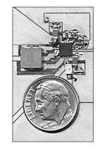
Figure 1. A typical LTC4001-based Li-Ion battery charger occupies minimal board real estate. by Tom Hack
