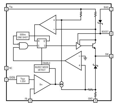
Figure 1. The block diagram of the LT3470 shows the integrated boost and catch Schottky diodes. Inductor current is kept under control at all times by monitoring the  $V_{IN}$  current as well as the catch diode current, thereby providing short circuit protection even if  $V_{IN} = 40V$ .
