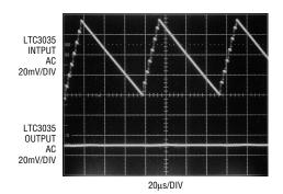
Figure 3. Input and output waveforms to the LTC3035 in the Li-Ion to 3.3V application, showing its excellent ripple rejection ( $I_{OUT}$  = 25mA, LTC3440 in Burst Mode<sup>®</sup>)
