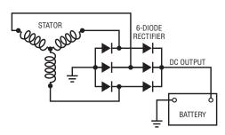
Figure 1. A standard alternator's 3-phase stator windings and 6-diode rectifier produce a DC output voltage.
