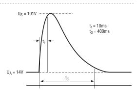
Figure 2. Unclamped load dump: If the battery connection is lost during charging, the alternator's output voltage can surge to 100V.
