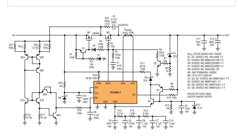
Figure 8. An LTC4380-based circuit protects downstream electronics from ISO 16750-2 and ISO 7637-2 transients while providing up to 4A of output current.
