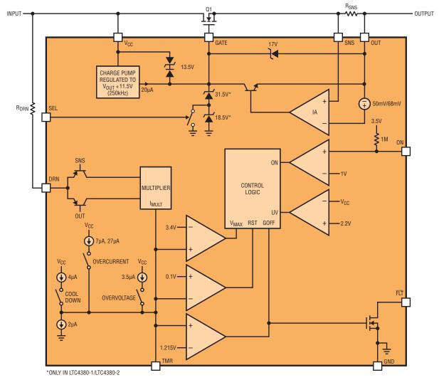
Figure 7. Block diagram of the LTC4380 surge stopper
