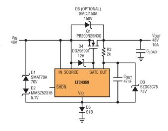
Figure 7. 48V ideal diode with reverse input protection
