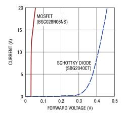
Figure 3. Load current vs forward voltage drop
