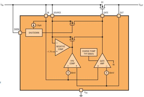
Figure 1. Block diagram of the LTC4359
