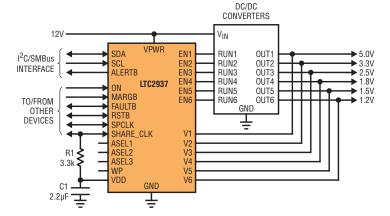
Each of the LTC2937's six channels has two dedicated comparators to accurately monitor over- and undervoltage conditions to within ±0.75%. The comparator thresholds are individually programmable over a range of 0.2V to 6V with 8-bit resolution.
