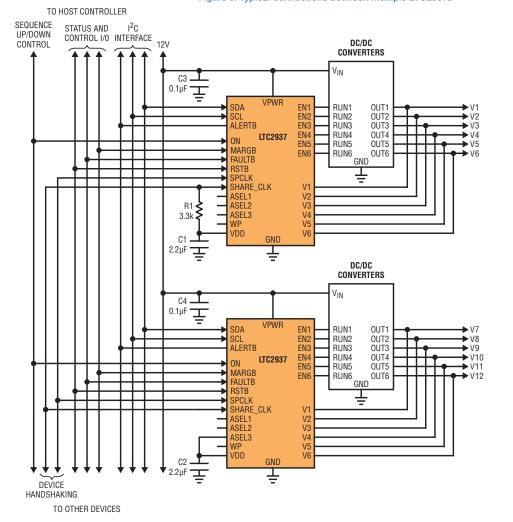
The LTC2937 simplifies power system sequencing and supervision. It requires very little board real estate for a complete system. It is flexible and reconfigurable, yet autonomous through its EEPROM memory. It can operate on its own, or in concert with other chips in a large system, seamlessly orchestrating the operations of up to 300 power supplies.
