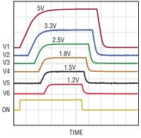
Figure 2. Power supply sequencing waveforms
