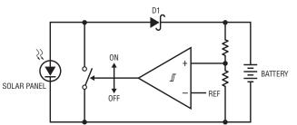
switch regulates battery charge in small solar system
