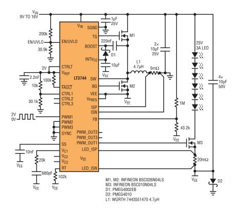
the anode of the high current LED is connected to ground to satisfy heat-sinking requirements. It is the floating  $V_{EE}$  feature that allows us to effectively use this part, originally designed for buck applications, as a synchronous boost mode LED driver.
