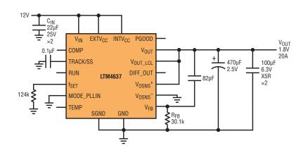
The LTM4637 is a complete POL power supply solution for applications that require top-notch performance in a small footprint with minimal design effort and user-adjustable feature versatility. Its low power loss and thermal resistance allow for up to 20A of load current per phase, while its current mode structure allows the load current to be scaled up via parallel configurations.
