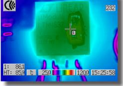
$T_{A} = 25^{\circ}C, \text{ NO AIR, NO HEAT SINK}$  $I_{LOAD} = 20A, V_{IN} = 12V, V_{OUT} = 1.8V$
