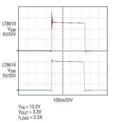
Figure 6. Dropout behavior of switch node for LT8614 and LT8610
