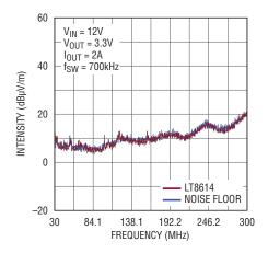
The LT8614 reduces EMI by more than 20dB when compared current state-of-the-art switching regulators. In comparison, it lowers EMI by 10x in the frequency range above 30MHz without compromising minimum on- and off-times or efficiency in an equivalent board area. It accomplishes this feat with no additional components or shielding, representing a significant breakthrough in switching regulator design.
