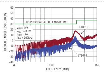
Figure 3. Comparison of radiated emissions for LT8614 and LT8610
