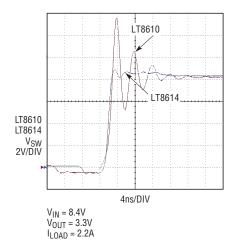
Figure 5. Near ideal square wave switch waveform of LT8614 enables low noise operation
