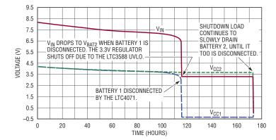
Figure 3. Discharge with battery undervoltage disconnect
