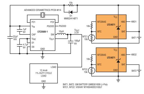
Figure 1. Complete piezo-based energy harvesting system is independent of the grid. This design uses thin film batteries to gather energy collected by the piezo for a wireless sensor transmitter, which operates on a 1% duty cycle. With a few easy-to-use components, it is possible to build a complete compact energy-harvesting power subsystem for wireless sensor-transmitters.
