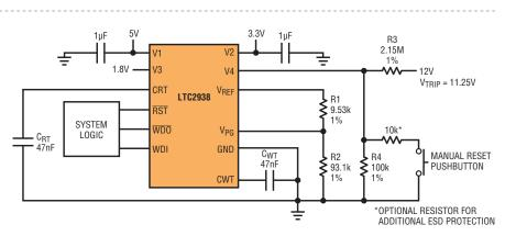
Figure 9. Quad-supply monitor (mode 14) with pushbutton reset
