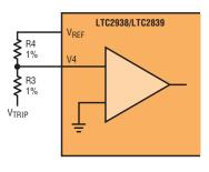
Figure 4. Setting the negative adjustable trip point,  $V_{TRIP} = -V_{REF} \bullet (R3/R4)$
