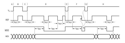
POWER-ON RESET FOLLOWED BY RESET CAUSED BY UNDERVOLTAGE EVENT. WATCHDOG OUTPUT SET HIGH, WATCHDOG INPUT = DON'T CARE WATCHDOG INPUT NOT TOGGLED, WATCHDOG TIMER EXPIRES, WATCHDOG OUTPUT PULLS LOW. RESET OUTPUT PULLS LOW FOR ONE RESET TIMEOUT PERIOD.
