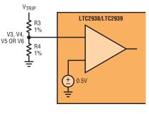
Figure 3. Setting the positive adjustable trip point, V<sub>TRIP</sub> = 0.5V • (1 + R3/R4)
