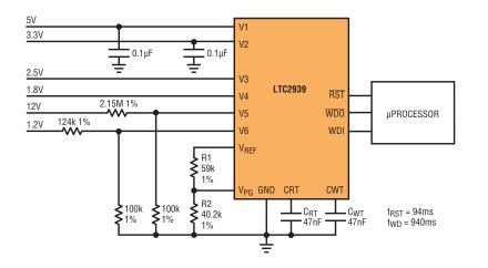
The LTC2938 and LTC2939 supply threshold voltages are configured by an external resistive divider from the  $v_{REF}$  pin to ground (see Figure 2). The center tap of the divider drives the  $v_{PG}$  pin. During power-up, the voltage at the  $v_{PG}$  pin is detected and used to select one of 16 possible configurations as shown in Table 1. Recommended ±1% resistor values to select each configuration can also be found in Table 1.
