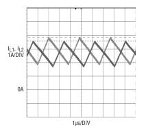
Figure 5. The inductor current in a 2-phase single output converter. Currents in both inductors shown with a 24V Input and 8.5V at 6A output.
