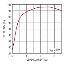
Figure 3. Efficiency of the converter in Figure 1 for the  $V_{OUT2}$  8.5V channel
