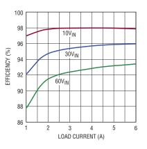
Figure 4. Efficiency of the LTC3890 configured as a 2-phase single output of 8.5V at up to 6A
