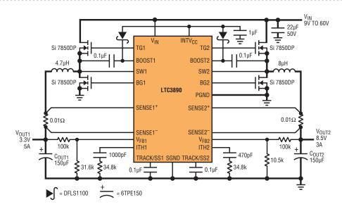
Figure 1. High efficiency dual 8.5V/3.3V output step-down converter
