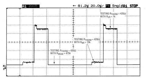
Figure 6. Testing an underrange thermistor
