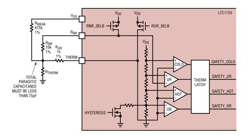
Figure 4. LTC1759 safety-signal-monitoring circuitry
