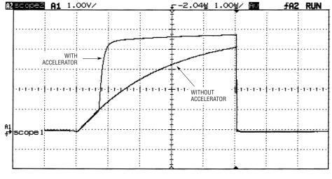
Figure 3. SMBus accelerator operation ( $R_{PULLUP} = 15k$ ,  $C_L = 150pF$ ,  $V_{DD} = 5V$ )
