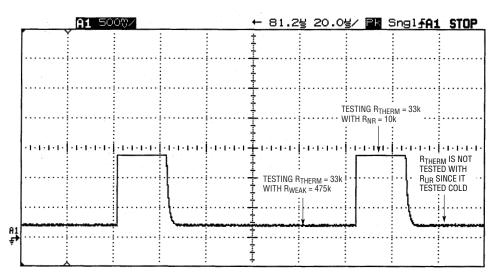
Figure 5. Testing a cold thermistor
