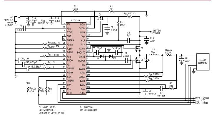
Shutdown of the PWM through the CHGEN–SDB pin combination occurs when the AC power is lost or the battery is removed. The LTC1759 detects the AC loss through the DCDIV pin. This threshold is usually set just below the lowest valid voltage of the wall adapter. AC power status may be read by the system over the SMBus. The UV pin is only used to put the PWM circuitry into micropower shutdown and is connected directly to the wall adapter supply.
