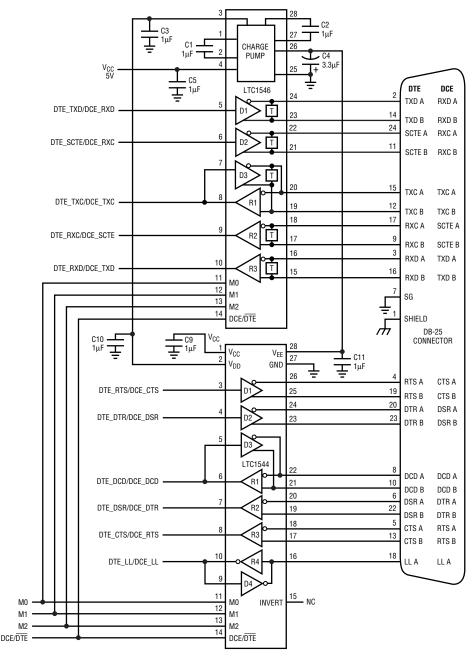
Figure 1. LTC1544/LTC1546 software-selectable multiprotocol DCE/DTE port
