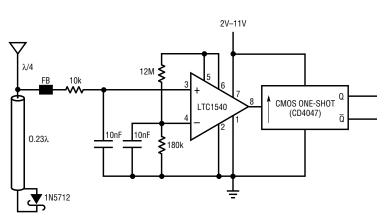
Figure 1. Nanopower field detector
