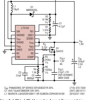
Figure 2. 1.8V to 1.5V, 4A very low dropout linear regulator (typical dropout voltage is 65mV at 4A)
