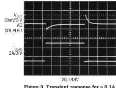
Figure 3. Transient response for a 0.1A to 4A output load step
