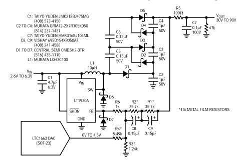
Figure 1. LT1930A-based boost regulator produces 30V to 90V for avalanche photodiode bias supplies with only  $200\mu V_{P,P}$  noise.
