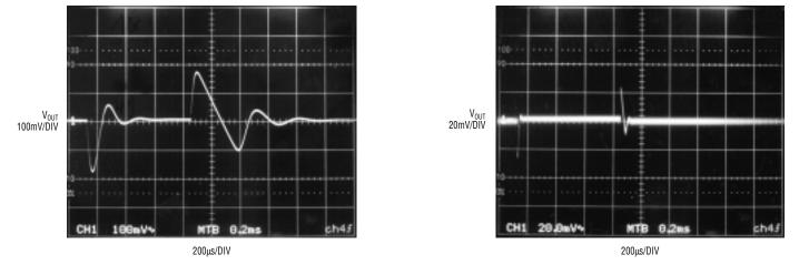
Figure 10. Before and after photos show dramatic improvement in transient response after the addition of a  $0.01\mu$ F bypass capacitor. Note the change in voltage scale
