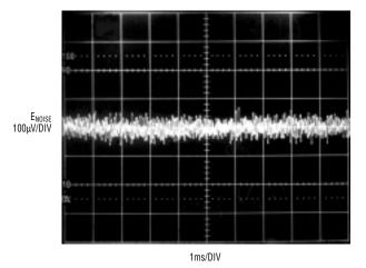
Figure 5. LT1761-5 output voltage noise
