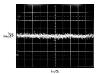
Figure 7. LT1761-BYP output voltage noise ( $V_{OUT} = 1.22V$ )
