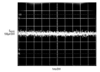
Figure 6. LT1761-3.3 output voltage noise
