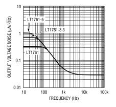
Figure 9. LT1761 noise spectral density
