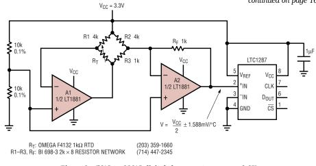
Figure 9. -50°C to 600°C digital thermometer runs on 3.3V
