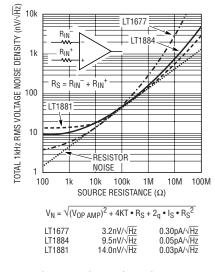
Figure 7. 1kHz noise voltage vs source resistance
