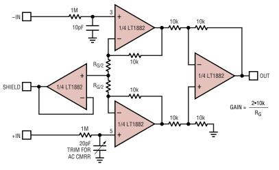
Figure 8. Input-fault-protected instrumentation amplifier
