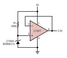
Figure 5. 2.5V reference from a 5V supply
