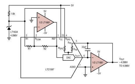
Figure 10. 16-bit voltage-output DAC on a  $\pm 5V$  supply
