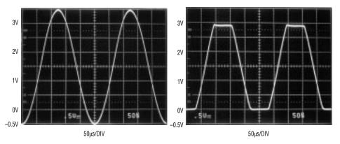
Figure 1. Input (left) and output (right) of an LT1677 configured as a voltage follower with input exceeding the supply voltage ( $V_s = 3V$ , input = -0.5V to 3.5V)
