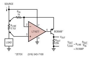
Figure 6. Precision high-side current sense amplifier
