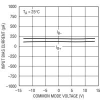
Figure 2. LT1884 input bias current vs common mode voltage
