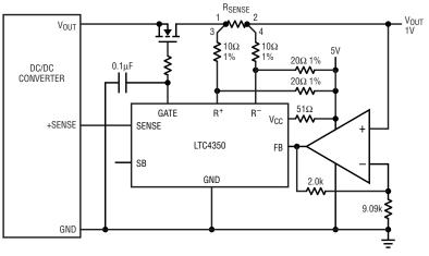
Figure 6. Example of 1V load share implementation (one channel)
