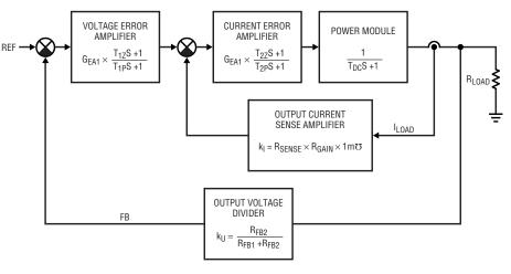
Figure 2. Power channel control system block diagram
