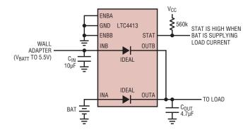
Figure 1. Automatic power switch between a battery and a wall adapter
