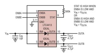
Figure 5. Dual high side power switch
