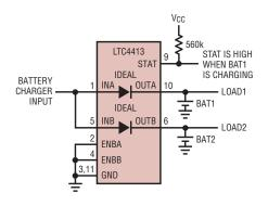
Figure 4. Multiple battery charging
