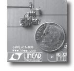
Figure 5. Photograph of demo board of circuit in Figure 4—board area is 10mm × 12mm
