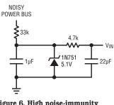
Figure 6. High noise-immunity input network allows 50V transients on automotive power bus.
