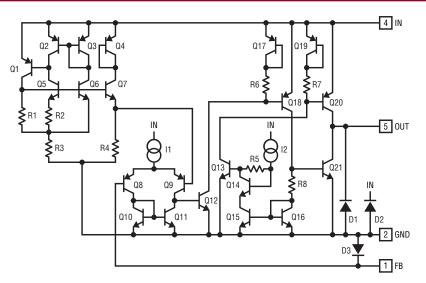
Figure 2. LT6650 simplified schematic showing detail of low-dropout topology
