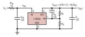
Figure 4. Simple input network for improved supply rejection
