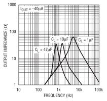
Figure 7. Output impedance is reduced while sourcing moderate current (40µA).
