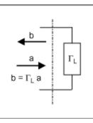
Figure 1-2a. Load flow graph.
