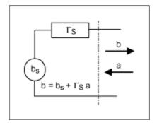
*Figure 1-3a. Power source reflection coefficient.*
