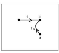
*Figure 1-3b. Power source flow graph.*
