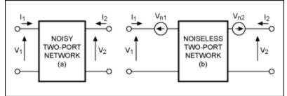
Figure 1. A noisy two-port network (a) can be modeled by a noise-free two-port network (b) with external noise voltage sources  $V_{n1}$  and  $V_{n2}$ .
