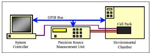
Figure 4. Cell characterization system.
