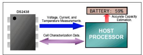
Figure 1. System diagram.
