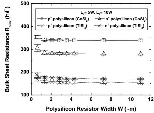
Figure 2. The relationship between the bulk sheet resistance (R<sub>bulk</sub>) and the polysilicon resistor width W with the polysilicon resistor lengths of L<sub>1</sub>= 5W and L<sub>2</sub>= 10W
