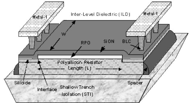
Figure 1. The schematic diagram of a polysilicon resistor
