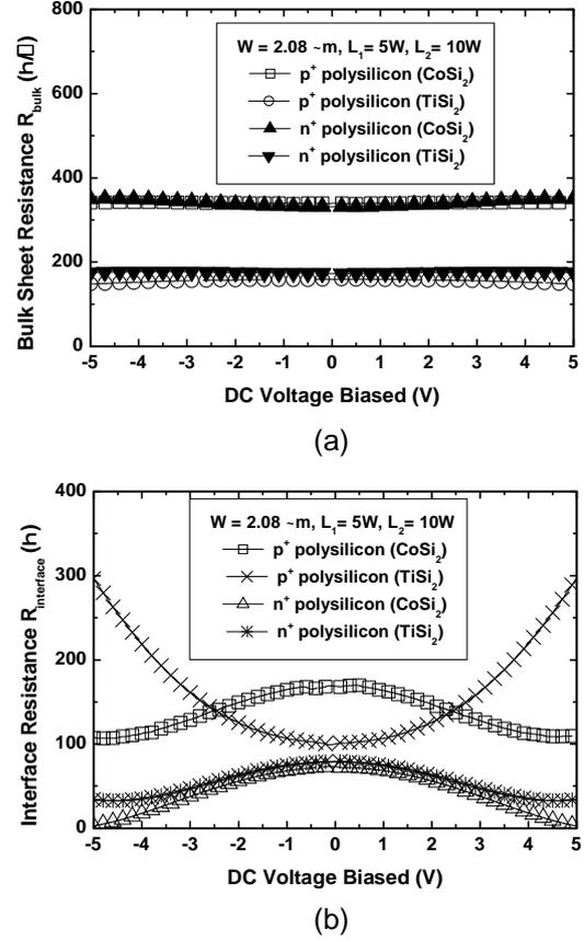
Figure 4. The voltage-dependent characteristics of (a)  $R_{\text{bulk}}$  and (b)  $R_{\text{interface}}$  with polysilicon resistor width  $W$  of  $2.08 \mu\text{m}$  of  $n^+$  and  $p^+$  polysilicons with Ti- and Co-silicide
