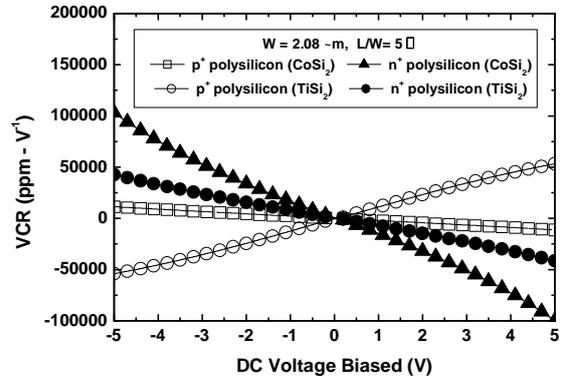
Figure 5. The VCR characteristics of Ti- and Co-silicide of  $n^+$  and  $p^+$  polysilicons with polysilicon resistor width  $W$  of  $2.08 \mu\text{m}$  and square number of  $5 \square$
