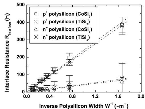
Figure 3. The relationship between the interface resistance R<sub>interface</sub> and the inverse polysilicon resistor width W<sup>-1</sup>
