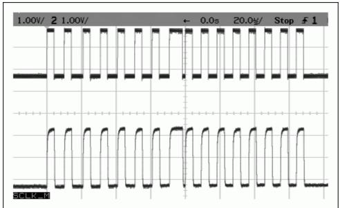
Figure 7. The SPI SCLK signal on both sides of the isolated interface. Top:  $ISOV_{CC} = 8.3V$ , ISOGND = 5V. Bottom: Powered by USB:  $V_{CC} = 3.3V$ , GND = 0V.
