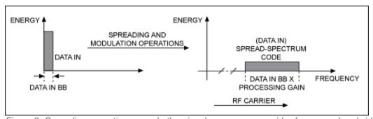
Figure 2. Spreading operation spreads the signal energy over a wider frequency bandwidth.
