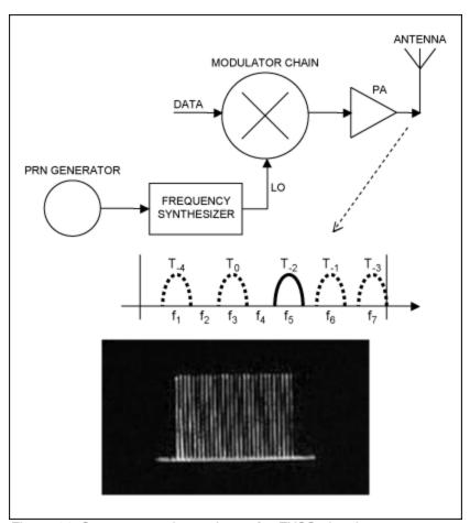
Figure 14. Spectrum-analyzer photo of a FHSS signal.
