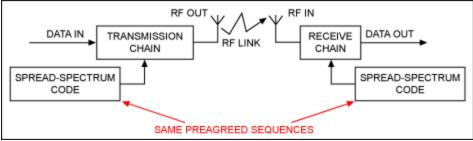
Figure 1. Spread-spectrum communication system.
