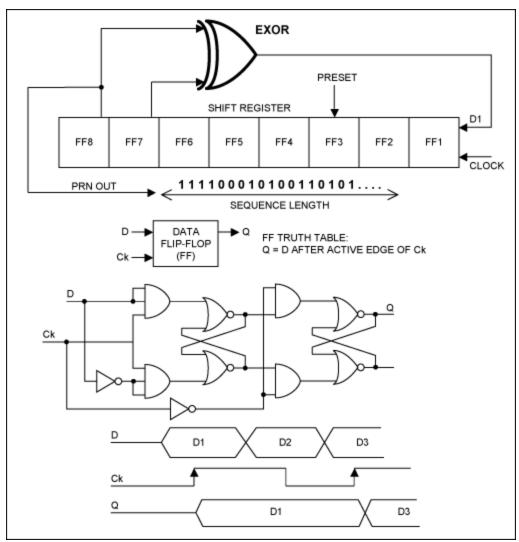
Figure 11. Block diagram of a sample PRN generator.
