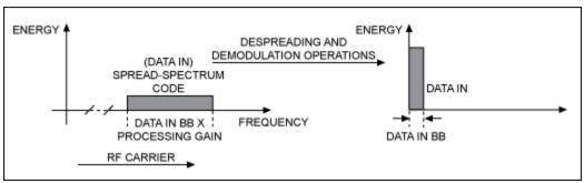
Figure 3. The despreading operation recovers the original signal.
