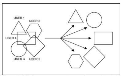
Figure 10. CDMA systems access the same frequency band with unique keys or codes.
