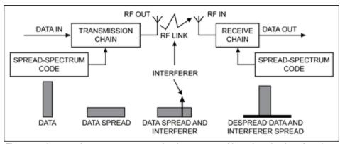
Figure 5. A spread-spectrum communication system. Note that the interferer's energy is spread while the data signal is despread in the receive chain.
