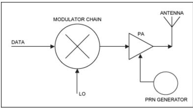
Figure 15. THSS block diagram.
